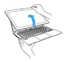
**3** Keep the LCD screen facing upward and pull the LCD screen lid in the direction of the arrow to place it over the keyboard.
