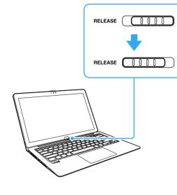
Once you slid the display release switch to RELEASE, it is locked and you cannot slide it back to the original position by hand.
