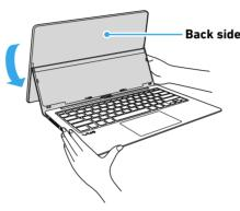
Turning the LCD screen lid lets the display release switch slide back to the original position.
