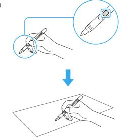
Alternatively, you can keep pressing the tip of the pen gently on the desired point for a few seconds to perform right-clicking.
