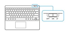
The Caps Lock indicator above the Caps Lock key and the → C charge indicator at the top right corner light for a fraction of a second and the keyboard turns on.
